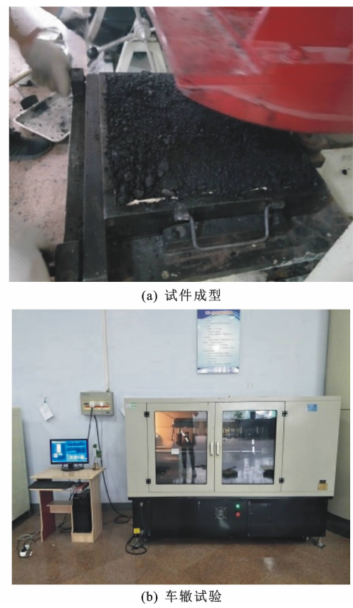
图 2 试件成型及车辙试验 Fig. 2 Molding specimen and wheel tracking test
