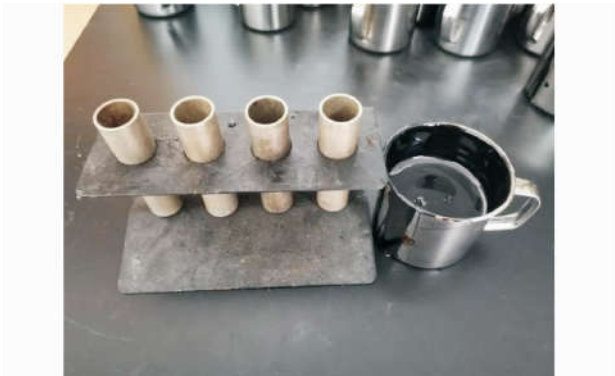
图 4 装有沥青胶浆试样的盛样筒 Fig. 4 Samples holder holding with asphalt mortar
