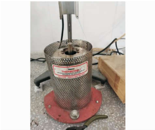
图 5 转子插入试样筒 Fig. 5 Put rotor into sample holder
