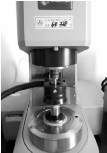
图2 DSR 震荡加载试验 Fig.2 DSR shock loading test
