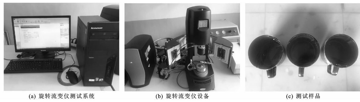
图 3 旋转流变仪及样品制备 Fig. 3 Rheometer instrument and sample preparation
