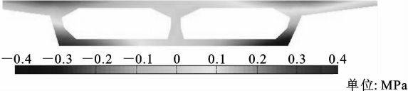
图 8 截面 1 箱梁在约束扭转时 x=6.0 m 处正应力分布 Fig. 8 Normal stresses distributions of box girder at x=6.0 m due to non-uniform torsion (section 1)
