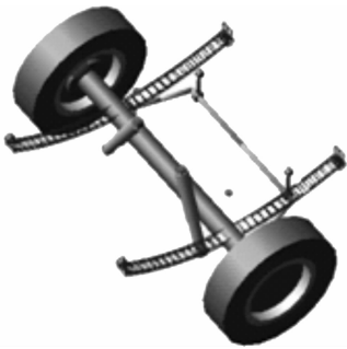
图 4 两片钢板弹簧后悬架多体模型 Fig. 4 Multi-body dynamic model of rear suspension with two paper leaf spring
