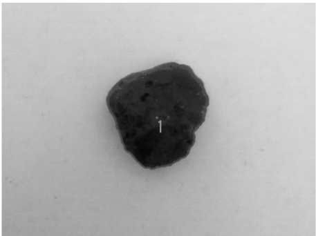
图 2 集料投影面形状提取 Fig. 2 Shape extraction of aggregate projection surface
