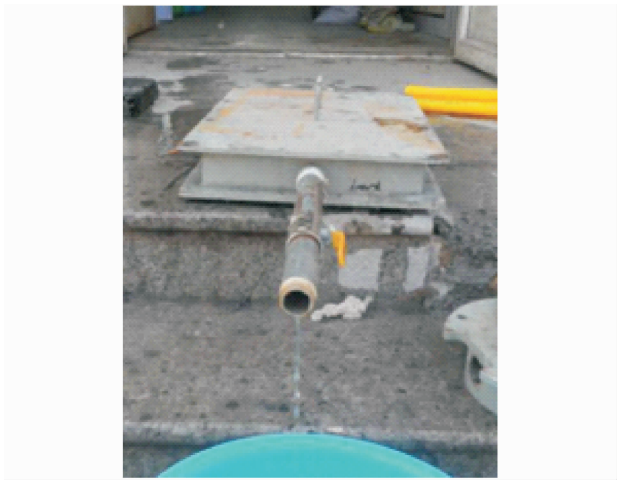
图 8 横向渗水系数测试 Fig. 8 Testing of transverse permeability coefficient
