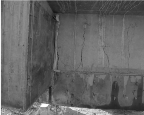
图 9 T2 梁弯曲破坏形态 Fig. 9 Flexural failure mode of girder T2
